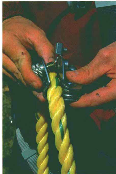
Rope grabs slide freely but stop sliding under weight. The stainless-steel rope grab connects the lanyard to the lifeline and automatically slides upward when the user ascends. To descend, the worker holds the locking mechanism lever in an upward position so that the cam lock rides freely as he lowers himself. The mechanism grabs the rope if the user slips.
