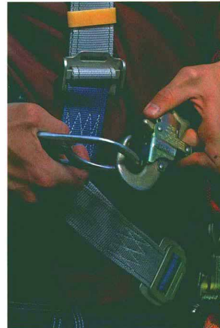
Here's a better way to hook lanyard to harness. It's always awkward and often difficult to reach behind the back and hook a lanyard to the D-ring that's attached to the body harness. This way works better. A 1-ft. lanyard that contains a shock absorber is factory-attached to the back of the harness, which can be swung around for attachment to a lanyard.
